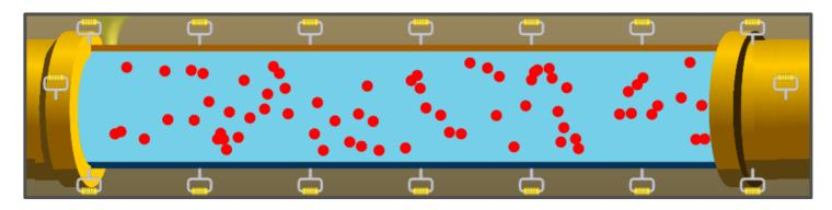
In the current simulation, the volume flow rate is 5000 L/s, or  $5 \text{ m}^3/\text{s}$ . This means that 5 cubic meters of water are passing through the pipe in a second. If the density of this water is  $1000 \text{ kg/m}^3$ , answer the following questions.
